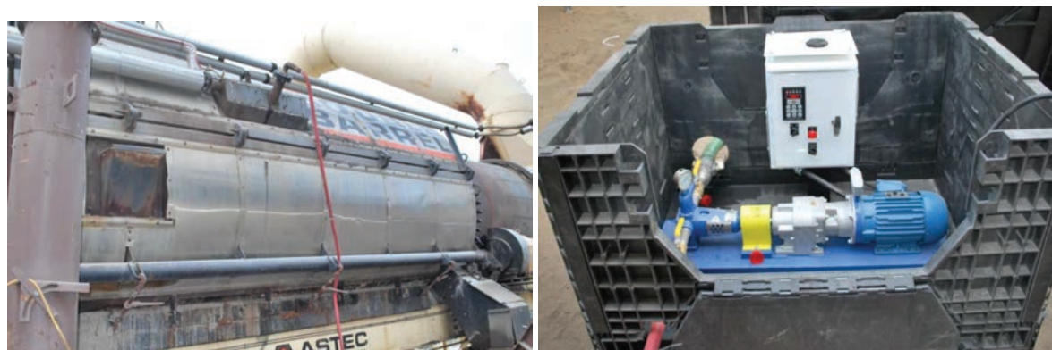
Figure C.10: Recycling agent injected to the binder line (left) and pump used to regulate the recycling agent dosage (right).
