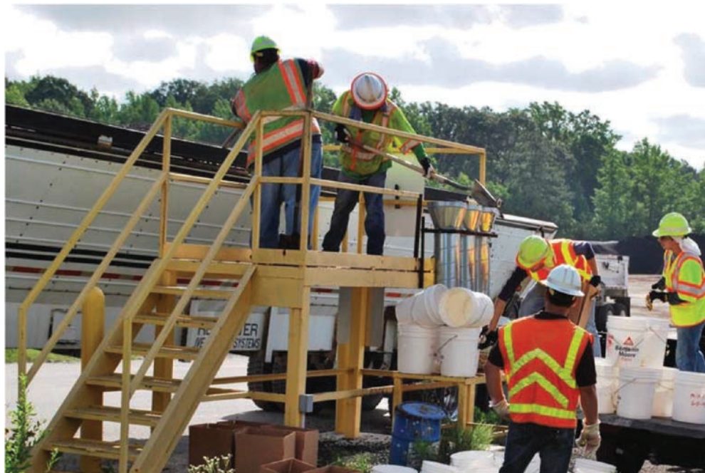
Figure A.15: Collection of Loose Mix from Truck at Asphalt Mix Plant.
