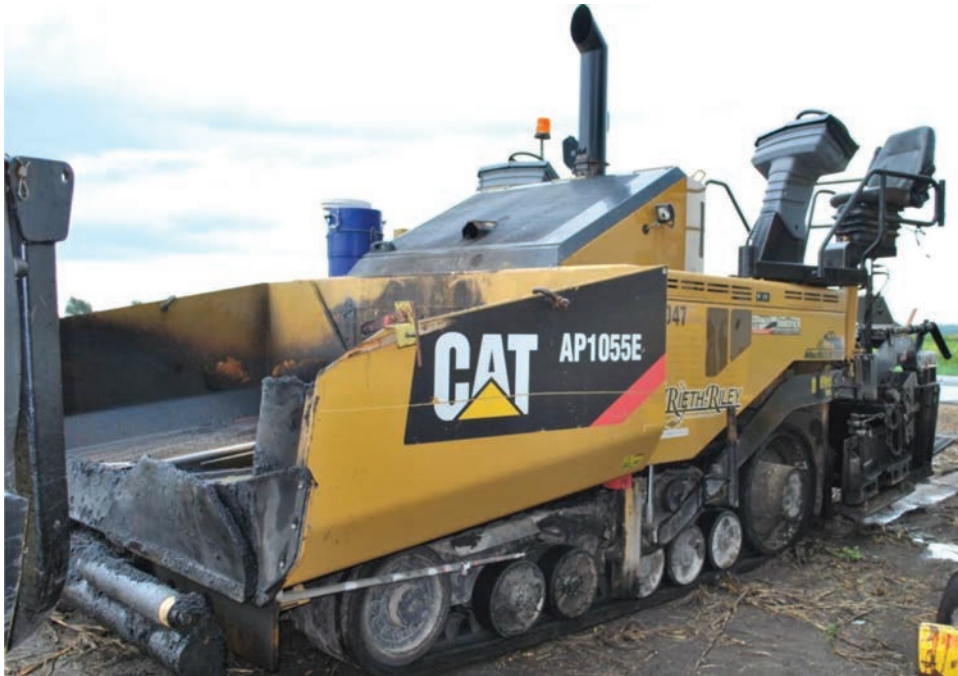
Figure C.12: Paver used for laydown at the Indiana field project.
