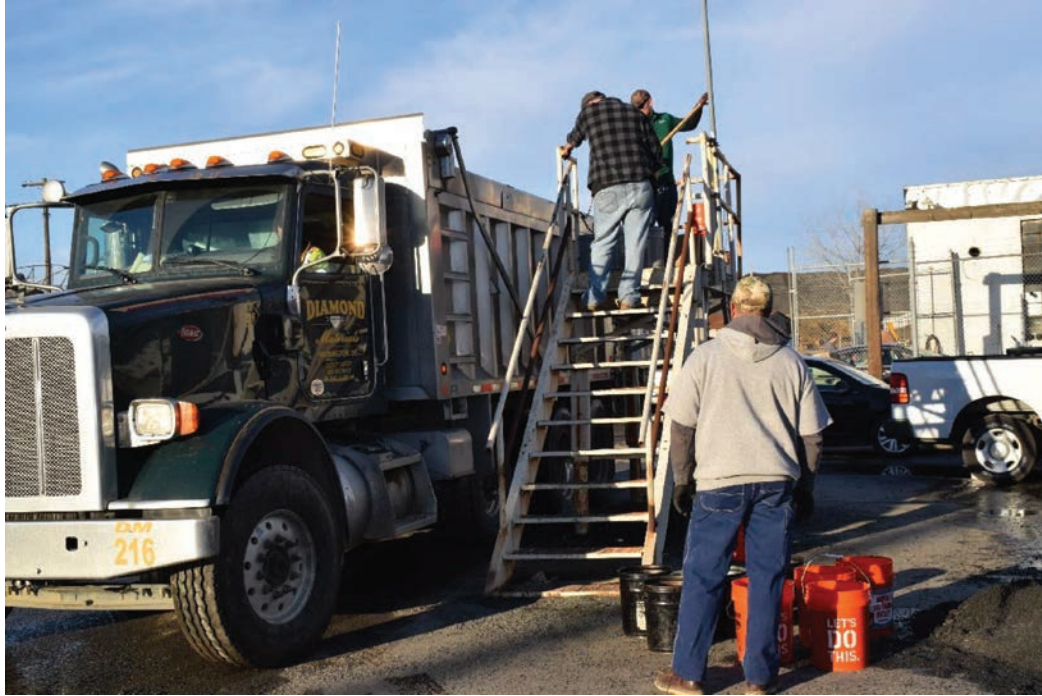
Figure E.13: Collection of Loose Plant Mix.
