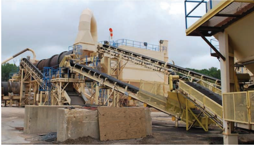
Figure A.16: Aggregate and RAP/RAS on Separate Conveyor Belts.
