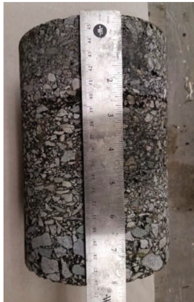
Figure E.3: Typical Full Depth Field Core.
