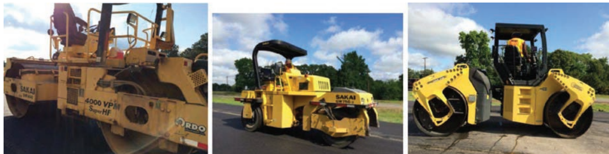
(a) Vibratory Roller
