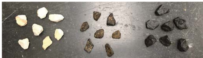
Figure 6. Coatability results for various recycling-agent incorporation methods: virgin aggregate (left), aggregates after replacing the base binder by the full recycling-agent amount (middle), and aggregates with no replacement of the base binder (right).
