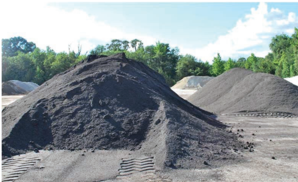
Figure A.18: RAS Stockpile.
